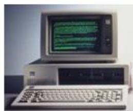
FOURTH-GENERATION COMPUTERS Fourth-generation computers, such as the original IBM PC shown here, are based on microprocessors. Most of today's computers fall into this category.
