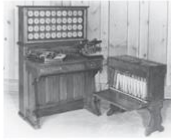
PRECOMPUTERS AND EARLY COMPUTERS Dr. Herman Hollerith's Punch Card Tabulating Machine and Sorter is an example of an early computing device. It was used to process the 1890 U.S. Census data.
