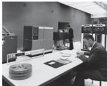
SECOND-GENERATION COMPUTERS Second-generation computers, such as the IBM 1401 mainframe shown here, used transistors instead of vacuum tubes so they were smaller, faster, and more reliable than first-generation computers.
