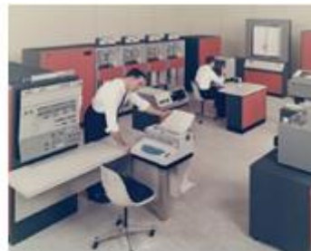
THIRD-GENERATION COMPUTERS Third-generation computers used integrated circuits, which allowed the introduction of smaller computers such as the IBM System/360 mainframe shown here.
